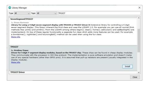
Once installed, open the included example by going to File > Examples > TM1637 > TM1637 test.
