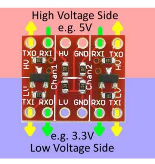
To send a signal from the low-voltage side to the high-voltage side (e.g. from 3.3 V to 5 V), the signal must be input at TXI. It will pass through the converter and come out as a higher voltage on the TXO (transmit output) pin.
