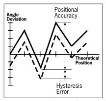
Figure 9. Positional accuracy of a stepper motor.
