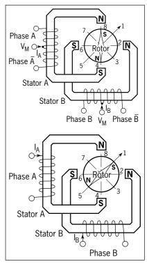
Figure 6. Unipolar and bipolar wound stepper motors.
