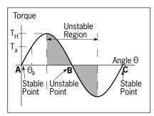
Figure 7. Torque vs. rotor angular position.
