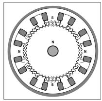
Figure 3. Cross-section of a hybrid stepper motor.
