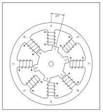
Figure 1. Cross-section of a variable-reluctance (VR) motor.
