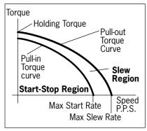
Figure 10. Torque vs. speed characteristics of a stepper motor.
