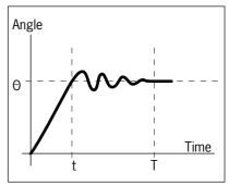
Figure 11. Single step response vs. time.
