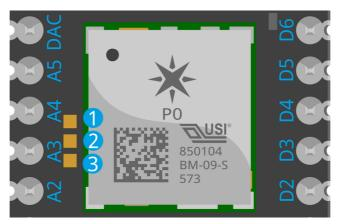
These pads would be used for the external coexistent interface to prevent simultaneous transmission on with an external radio, such as Bluetooth, while the Wi-Fi radio is transmitting. However the Wi-Fi radio software that runs on the P0, Broadcom/Cypress WICED, never supported this feature, so it cannot be enabled.
