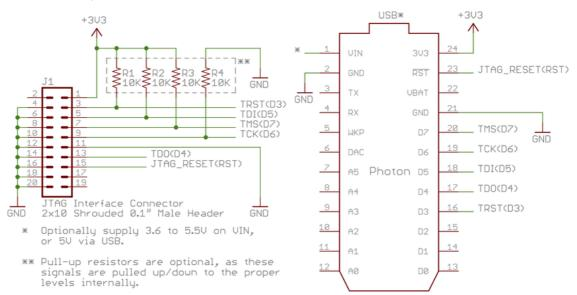
A standard 20-pin 0.1" shrouded male JTAG interface connector should be wired as follows:
